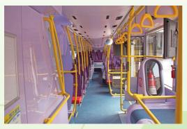
車廂設顏色鮮明及連貫性的扶手,由上車門位置伸延至車尾,方便視障人士進出車廂 Coherent handrails of high colour contrast are installed in bus compartment from front to rear for easy movement of the visually impaired
