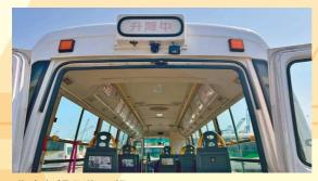
升降台操作指示燈 Warning signal during lift operation
